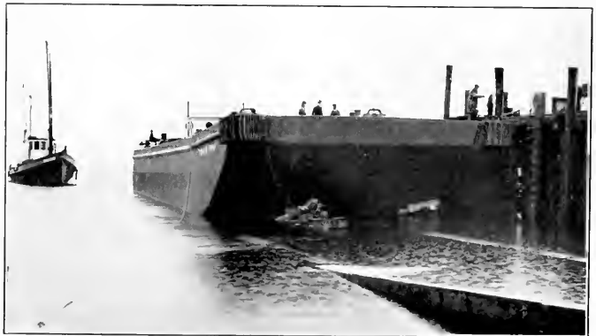
Steel oil barge recently completed by Lake Washington Shipyard for the Foss Tug and Barge Company of Seattle and Tacoma. This barge will be used around Puget Sound, transferring oil to the smaller ports, and is the first of its type to operate on the Sound. It has a capacity of 7500 barrels and is equipped with Northern pumps.
